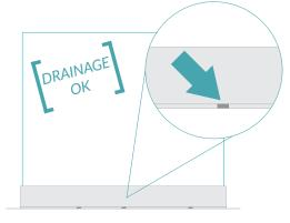
U-Channel Slim Base Shoe Track System with optional drainage profiles [side view]
