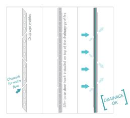
U-Channel Slim Base Shoe Track System with optional drainage profiles
