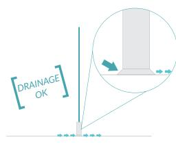
U-Channel Slim Base Shoe Track System with optional drainage profiles
